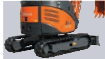
Two Travel Speeds Provided Two different travel speeds are available, making transport of the machine through the jobsite more efficient and smooth.
