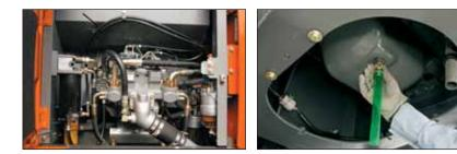
Wide doors give access, from ground level, to the fuel filter, water separator and engine oil filter. A large handrail, steps and anti-skid plates lead to the engine cover. The engine oil pan is fitted with a drain coupler. When draining, an associated drain hose is connected to the drain coupler. The drain coupler is reliable, avoiding oil leakage and vandalism.
