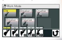
When replacing the attachment, oil flow adjustment can automatically be done by one touch on the work mode selection display on the LCD monitor. Minor adjustments of oil flow is possible if necessary.
