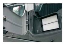
The fresh air filter for the air conditioner is relocated to cab door side from conventional location behind the operator seat. This allows easy cleaning and replacement of the fresh air filter, like the air circulation filter inside the cab.
