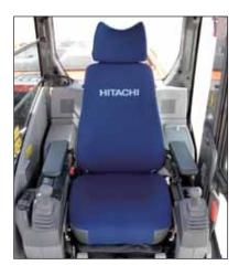
Wide adjustable armrests and a retractable seat belt are included. Short stroke levers allow for continuous operation with less fatigue. Three switches on the lever (optional) can be set to operate attachments other than buckets. The cab is pressurized to keep out dust. Noise and vibrations are kept to a minimum due to the elastic mounts, filled with silicone oil, the cab rests on.
