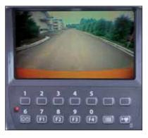
The widescreen color LCD, teamed up with the rear view camera on the counterweight provides rearward viewing.
