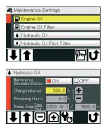
Replacement timing of hydraulic oil and fuel filters is alerted to the operator through the LCD monitor according to the schedule preset by the user each time when turning the key switch. The scheduled maintenance can prevent the failure of the machine. Attachment support system (work mode selector)
