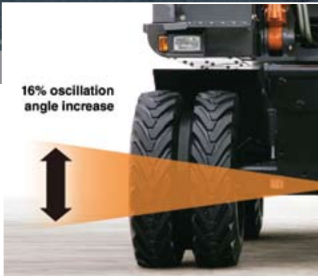
The oscillation angle has been increased by 16 percent over the conventional, improving surface holding performance on rough roads.
