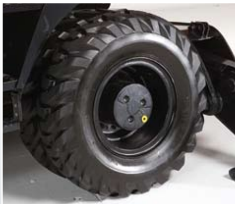
The tires feature an improved tread pattern and cross-section form, lowering vibration and noise while in motion.
